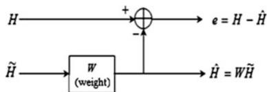
Fig. 2 Channel estimation using MMSE technique
